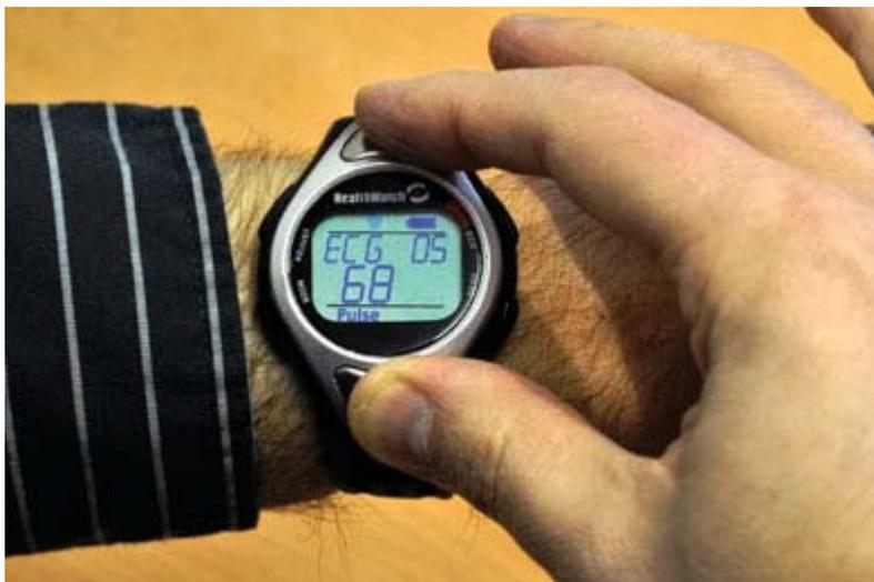
*The arrhythmia wristwatch can record a 1-lead ECG in 40 seconds*
